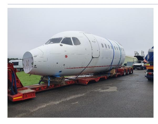
• Transported to Kemble Airport and open fuselage section blanked off
